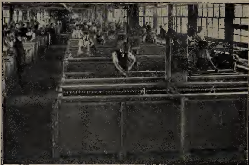
FIG. 192. The process of electroplating with nickel
